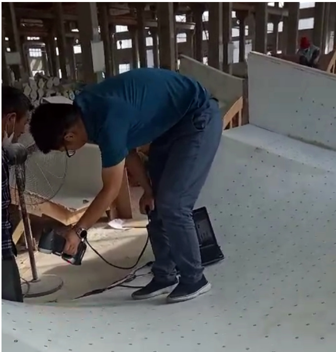
Figure 9. 3D-Scanning compare to the digital model.
